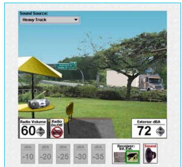
Vehicle passbys are heard for outdoors and indoors at different levels of sound insulation
